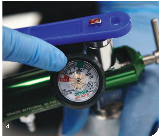
Figure 6-36, a-d: To attach the pressure regulator to the cylinder: a, insert the gasket into the pressure regulator; b, check to see that the pin index corresponds to the oxygen tank; c, seat the prongs of the regulator inside the cylinder and hand-tighten the screw until the regulator is snug; and d, turn on the oxygen and check how much pressure is in the cylinder.
