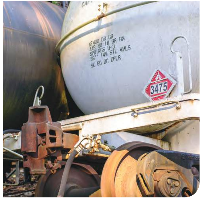
Figure 2-3: Hazardous material placard.
