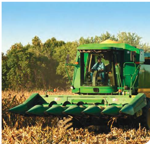
Figure 24-7: Combine parts, such as the auger, heads, reels, and snapping rollers, can cause serious injuries.
